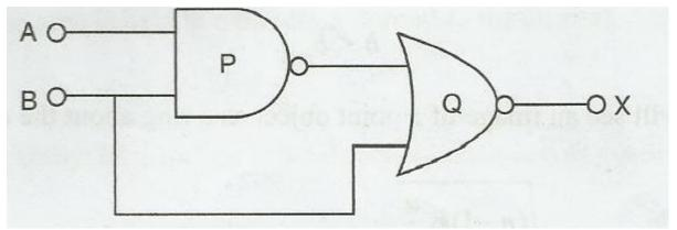
(ii) Write down the output at X for the inputs A=0 , B=0 and A=1 , B=1. Or
