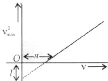
Light of frequency  $\nu$  is incident on a photosensitive surface. A graph of the square of the maximum speed of the electrons ( $V_{2\text{max}}$ ) vs.  $\nu$  is obtained as shown in the figure. Using Einstein's photoelectric equation, obtain expressions for
