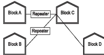
For layout 2, since the distance between Blocks A and C is large so a repeater would ideally be placed in between this path.
