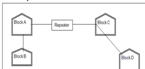
In both the layouts, a hub/switch each would be needed in all the blocks, to interconnect the group of cables from the different computers in each block
