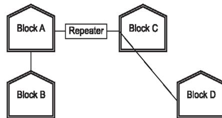
(ii) In both the layouts, a hub/switch each would be needed in all the blocks, to interconnect the group of cables from the different computers in each block.
