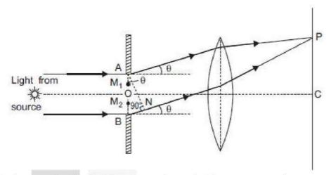
At the central point C of the screen, the angle  $\theta$  is zero. Hence the waves starting from all points of slit arrive in the same phase. This gives maximum intensity at the central point C. If point P on screen is such that the path difference between rays starting from edges A and B
