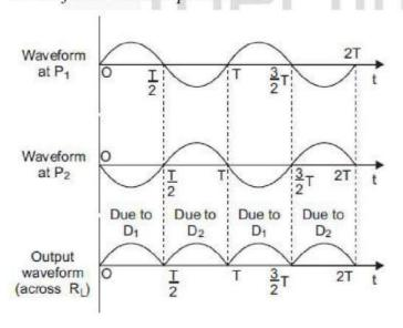
In a full wave rectifier, if input frequency is f hertz, then output frequency will be 2f hertz because for each cycle of input, two positive half cycles of output are obtained.
