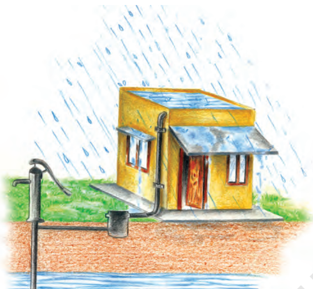
(a) Recharge through Hand Pump
