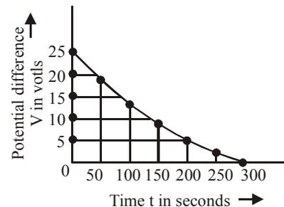
The figure shows an experimental plot for discharging of a capacitor in an R-C circuit. The time constant  $\tau$  of this circuit lies between:-
