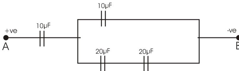
For supply  $V_{AB}=300$  V, determine the charge and voltage across each capacitor.
