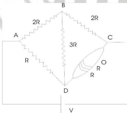
The resistance, of BC and CD arms, are now interchanged and another carbon resistor is connected in place of  $R$  so that the current through the arm BD is again zero. Write the sequence of colour bands of this carbon resistor. Also, find the value of current through it.
